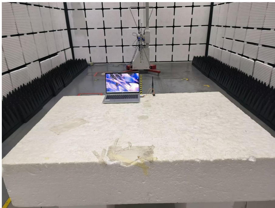
Radiated spurious emission Test Setup-1(Below 1GHz)
