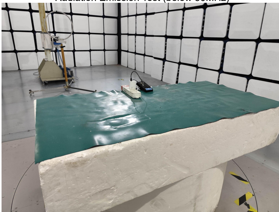
Radiation Emission Test (below 30MHz)
