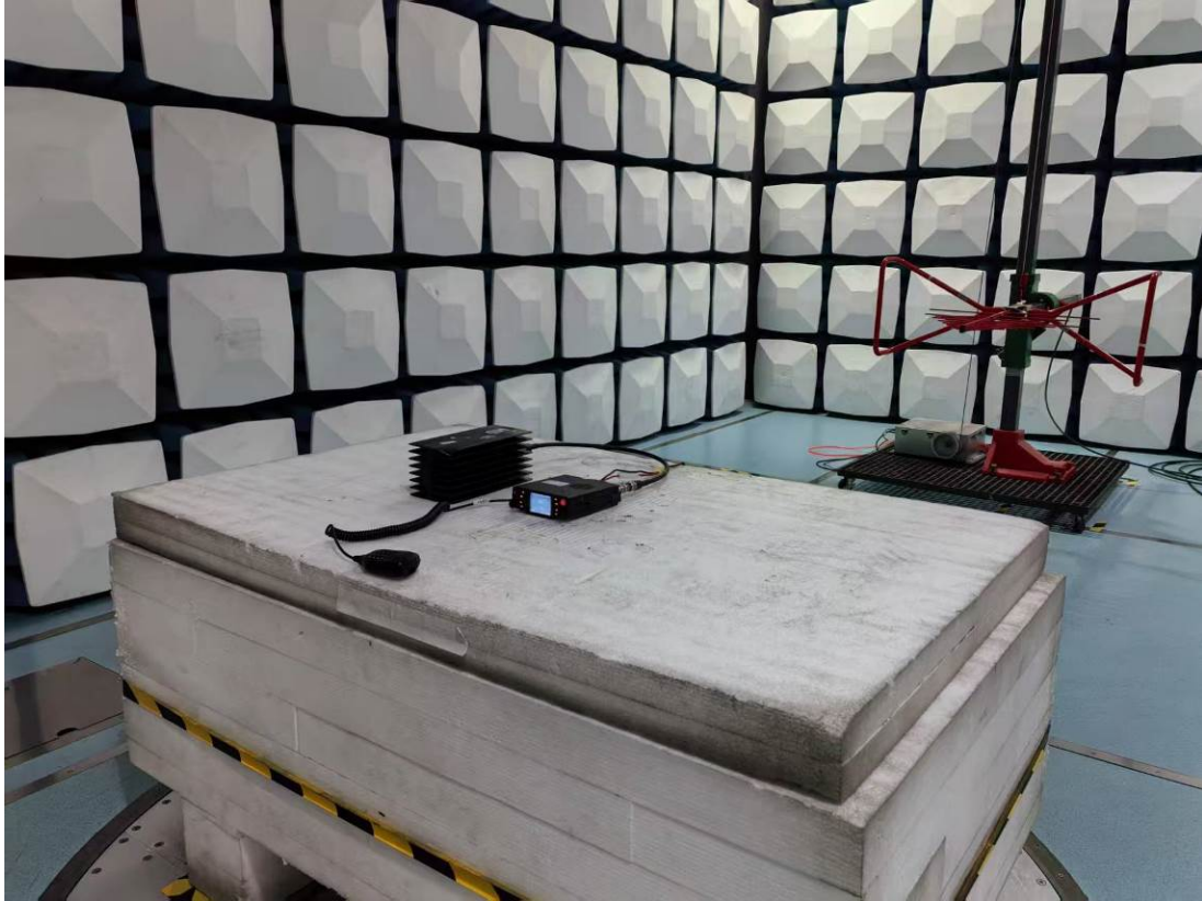
Radiated Emission Above 1GHz View
