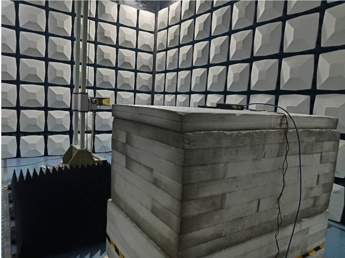
Radiated Emission Above 1GHz View
