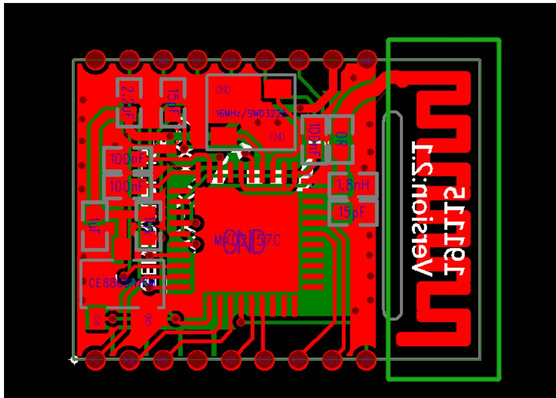
**Antenna Type:** PCB antenna
