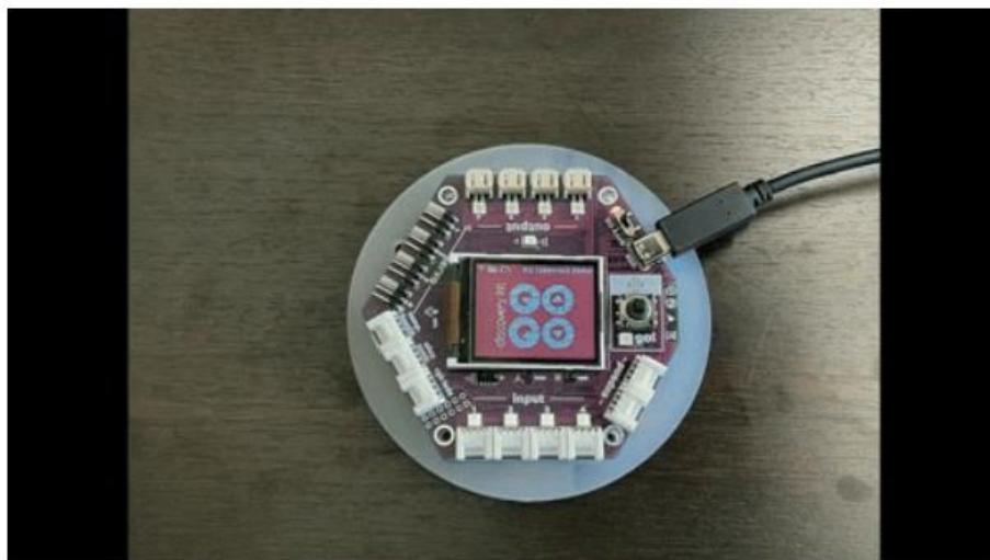
The GoGo Board is powered through a USB-C cable. The power source can be a computer or a power bank. After connecting the USB cable, slide the power switch next to the USB port to turn on the GoGo Board. You should see the screen turn on and hear a beep.
