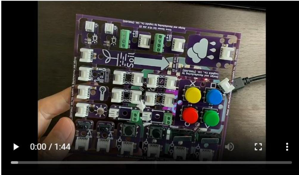
The GoGo Board uses Grove Sensors, many of which are included in the kit. To try, connect a sensor to one of the 4 input ports using a Grove cable. Use the joystick to navigate to the screen titled “Inputs”. You should see bar graphs with values that change depending on the sensor’s value.
