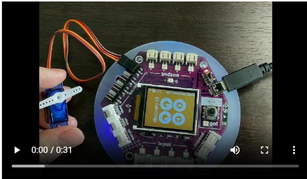
A Servo Motor is a kind of motor that turns only 180 degrees. The main benefit is that you can tell it where to point. Connect a Servo Motor to the Servo output port 1 and follow these steps:
