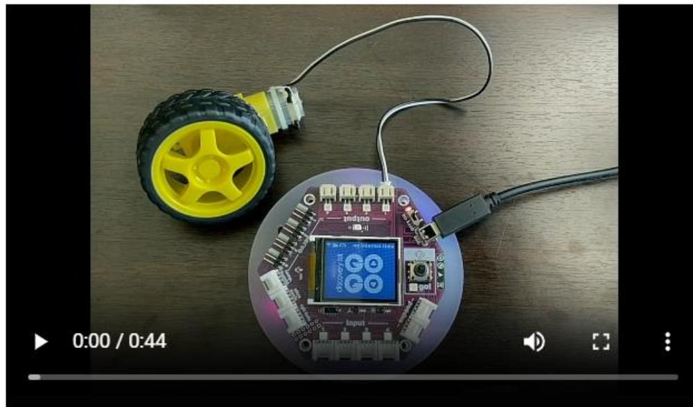
Connect a DC motor to output port 1. Then navigate the built-in screen using the joystick located on the right of the screen. Press down until you see the screen titled “Outputs”. Then control the motor by following these steps:
