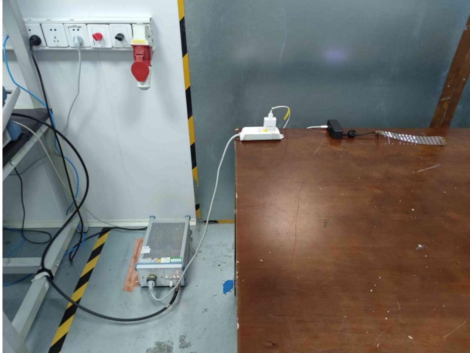
Conducted emissions at AC power line (150kHz-30MHz)
