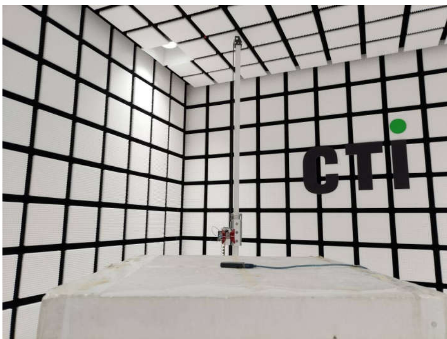
Radiated spurious emission Test Setup-2(Above 1GHz)
