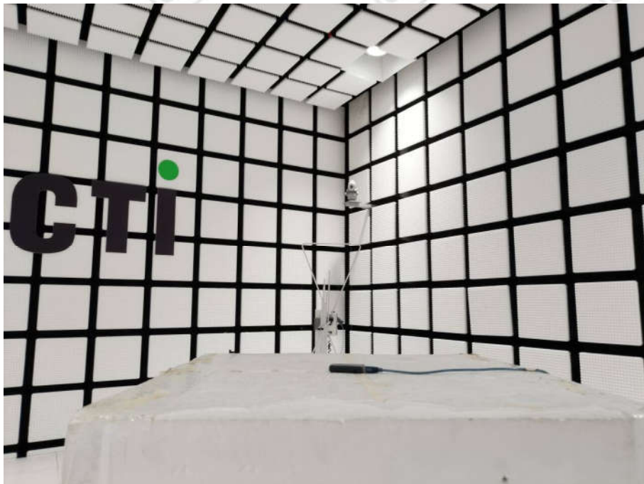
Radiated spurious emission Test Setup-1(Below 1GHz)
