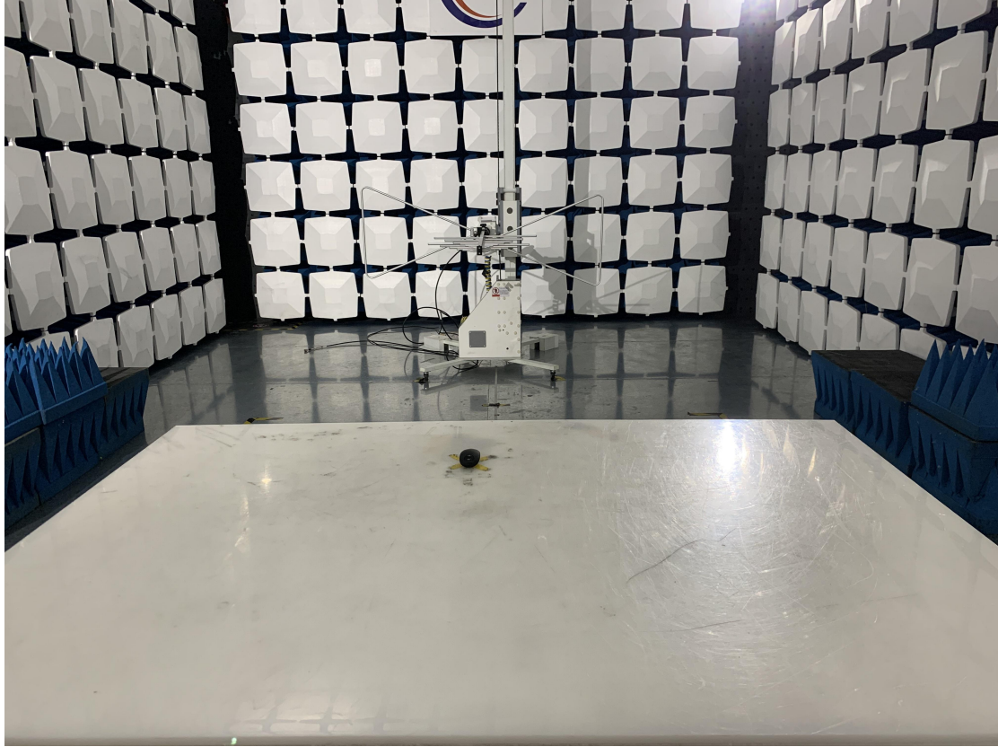
Above 1GHz for radiated emission test setup
