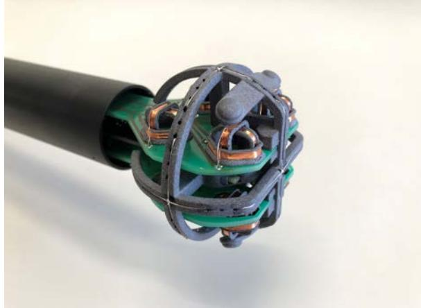
Test probe, without the casing
