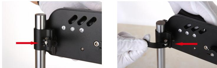
③This nut can adjust the tightness of the power clamp;
