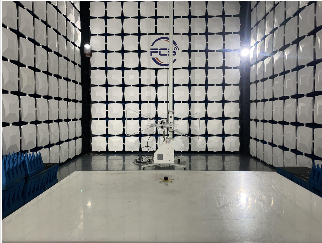
Above 1GHz for radiated emission test setup
