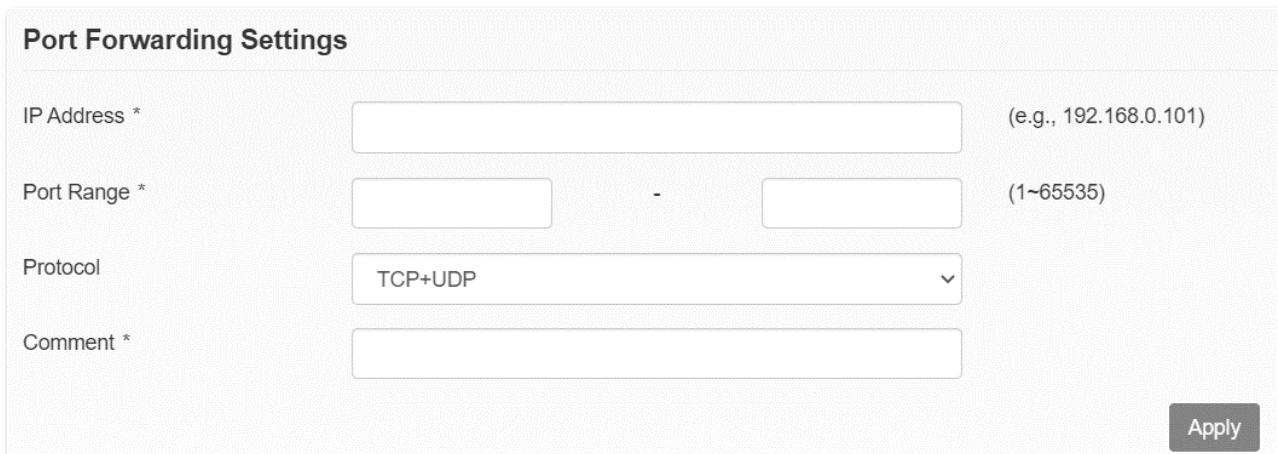
The screenshot shows the 'Port Forwarding Settings' page. It contains fields for 'IP Address \*' (with a placeholder '(e.g., 192.168.0.101)'), 'Port Range \*' (with a range from '1~65535'), 'Protocol' (set to 'TCP+UDP'), and 'Comment \*'. At the bottom right is an 'Apply' button.
