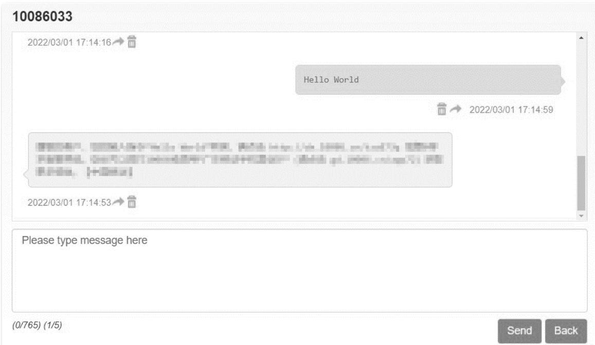
If the delivery report function on the SMS Settings module is enabled, a delivery message appears in the lower-right corner as well.
