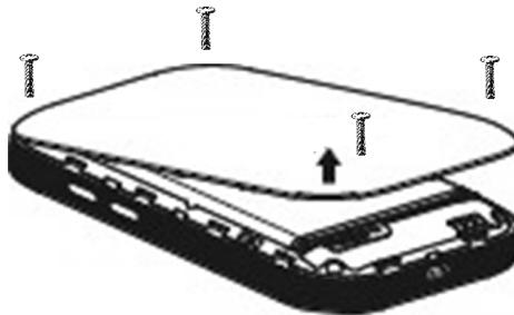
**Step 2** Slide and lift up the slot cover, insert a 3FF SIM card (an LTE, UMTS, or WCDMA SIM card) into the SIM card slot, and slide the cover back to lock.
