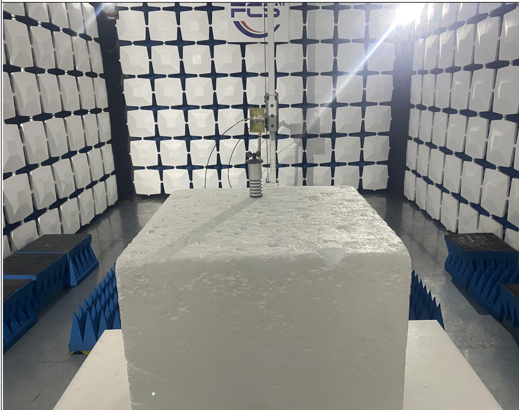
Above 1GHz for radiated emission test setup
