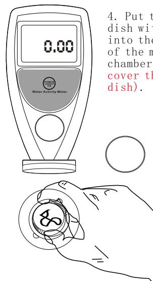
4. Put the container dish with sample into the bottom box of the measuring chamber (do not cover the container dish).
