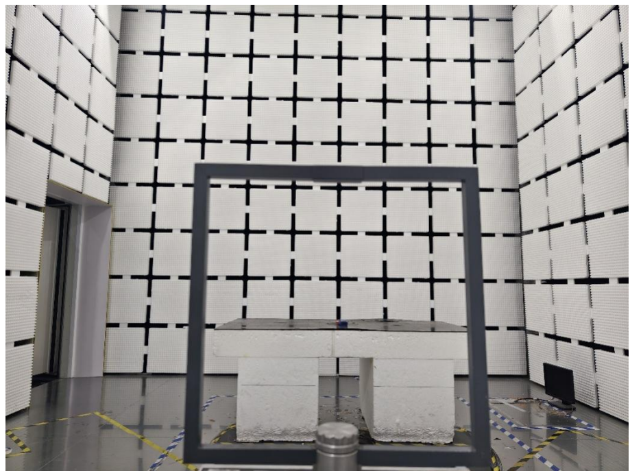
Radiation Emission Test Setup (Below 30MHz)
