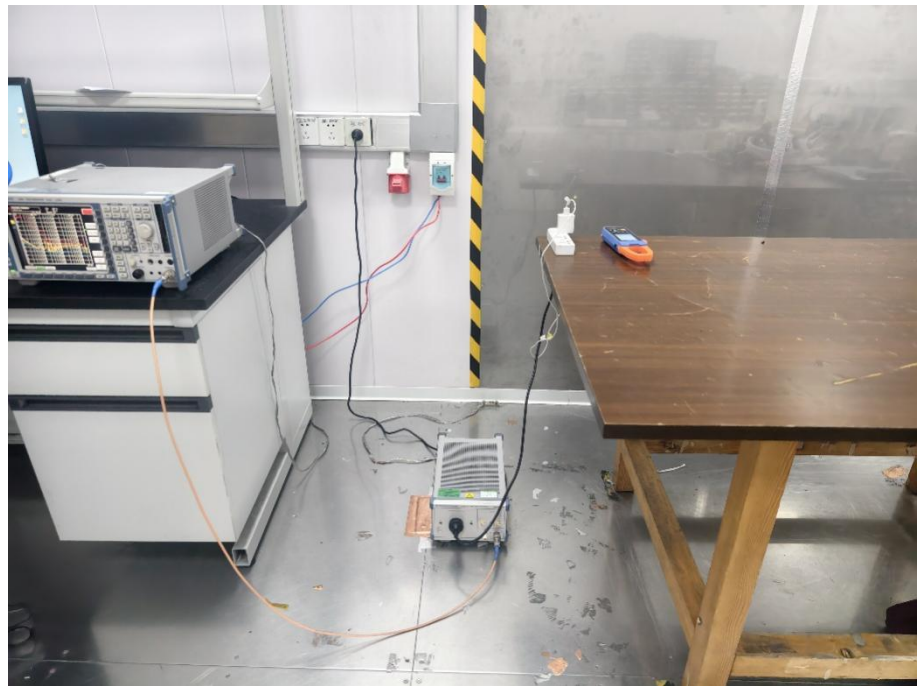
Conducted Emission Test Setup
