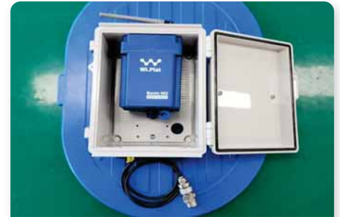
Sonic M2 Set (Main body, pressure sensor, device case)
