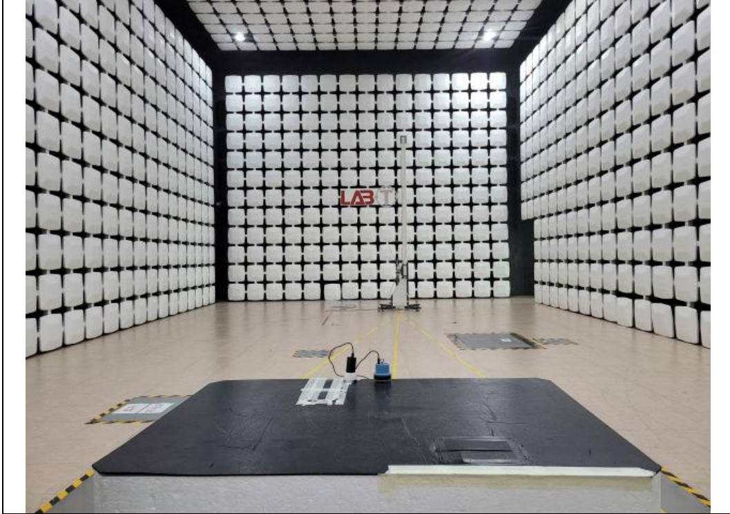
Radiated Emission (30 MHz to 1 000 MHz)_ Charge+Operating Mode Front
