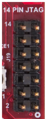
Figure 2-21. 14-Pin JTAG Connector
