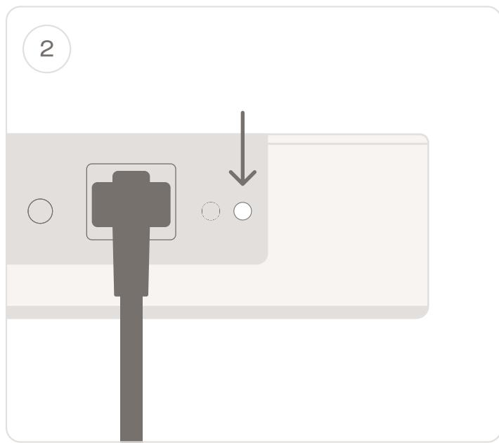
The sensor status LED will illuminate solid white once the device has booted and the radar is enabled.
