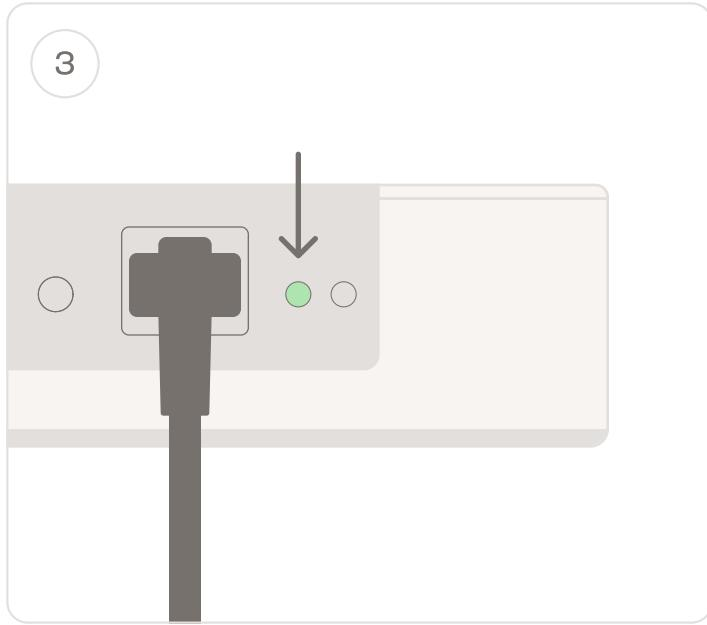
The connection status LED will slowly pulse green once the device is connected to the Gumband Cloud.
