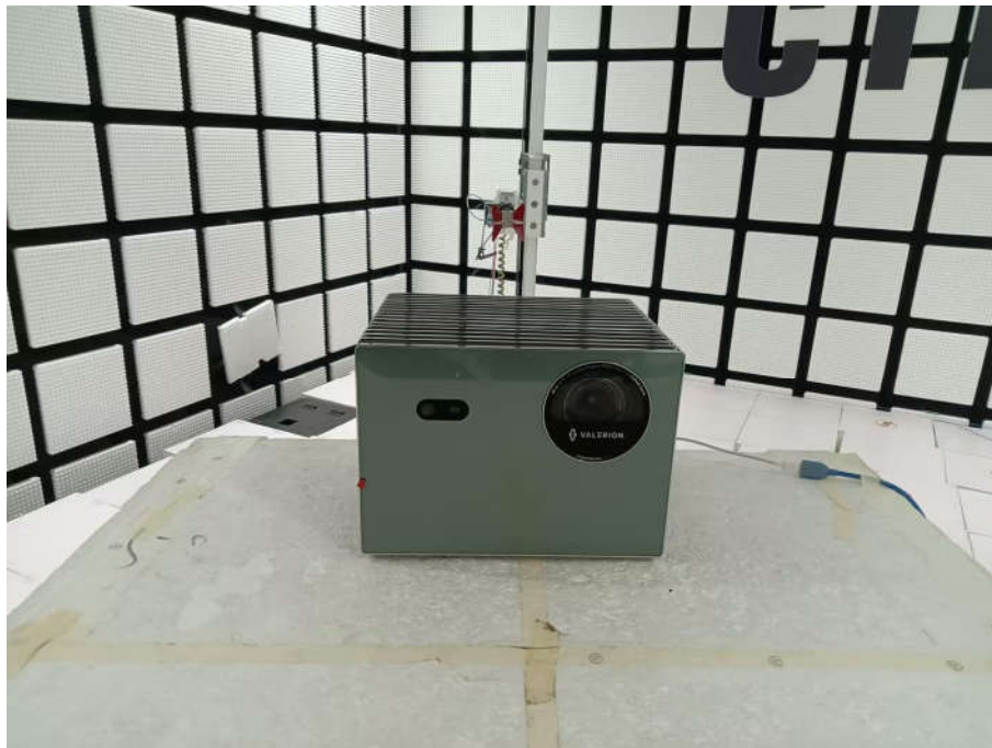
Radiated spurious emission Test Setup-3(Above 18GHz)
