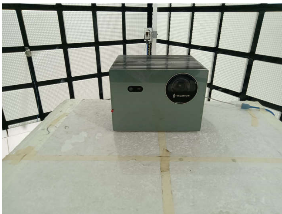
Radiated spurious emission Test Setup-2(Above 1GHz)
