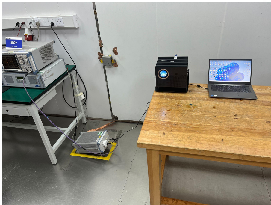
Conducted Emissions Test Setup
