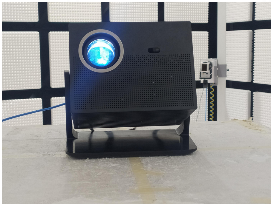
Radiated spurious emission Test Setup-3(Above 18GHz)
