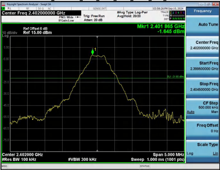
2 Spurious Emissions NVNT ANT1 1-DH1 2402 00
