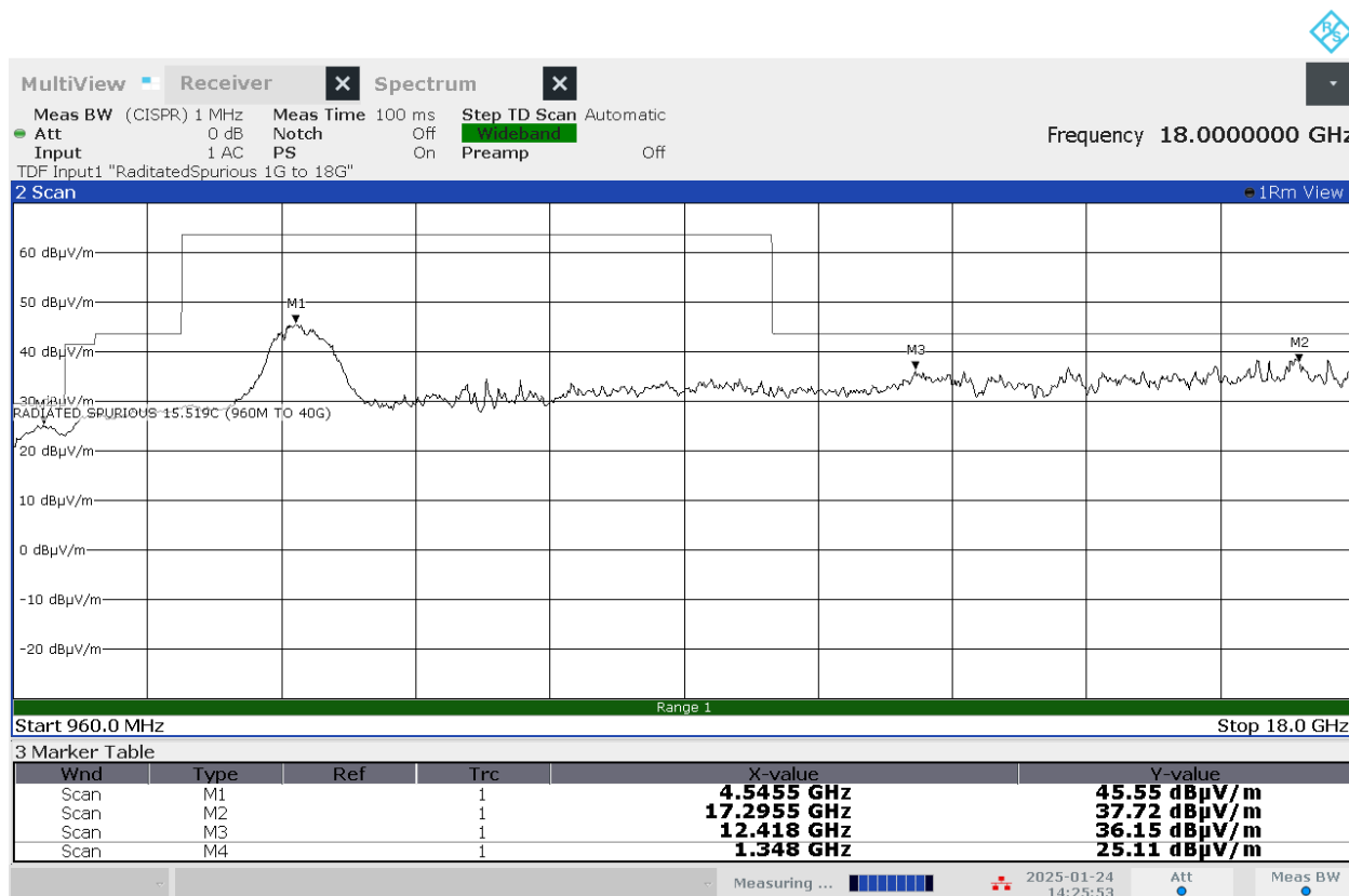
Figure 26. Radiated Emissions 960MHz – 18GHz (Vertical, Mid Channel)
