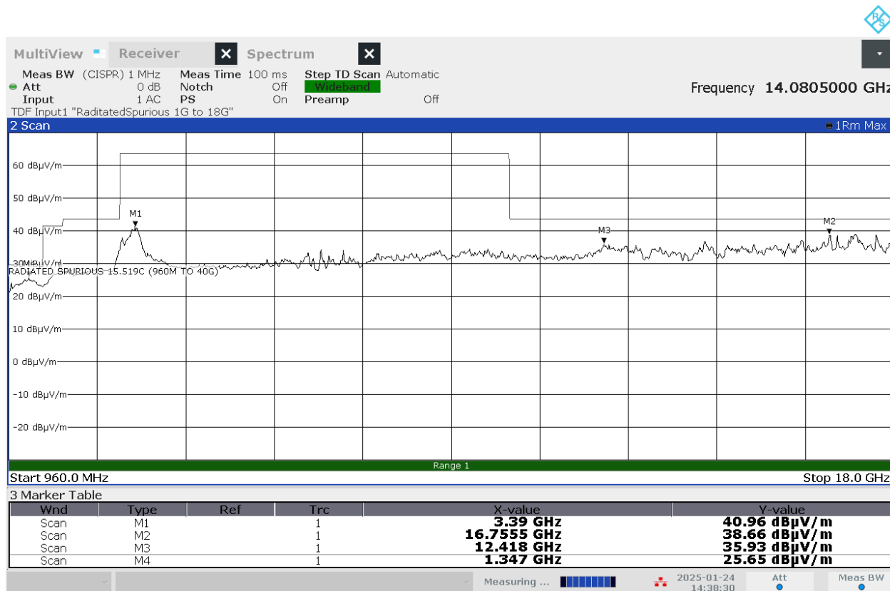
Figure 28. Radiated Emissions 960MHz – 18GHz (Vertical, High Channel)
