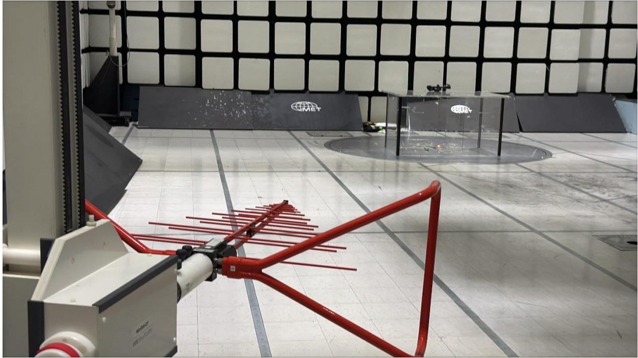
Radiated Emissions 30MHz – 1GHz (Antenna View) EUT at 80cm height
