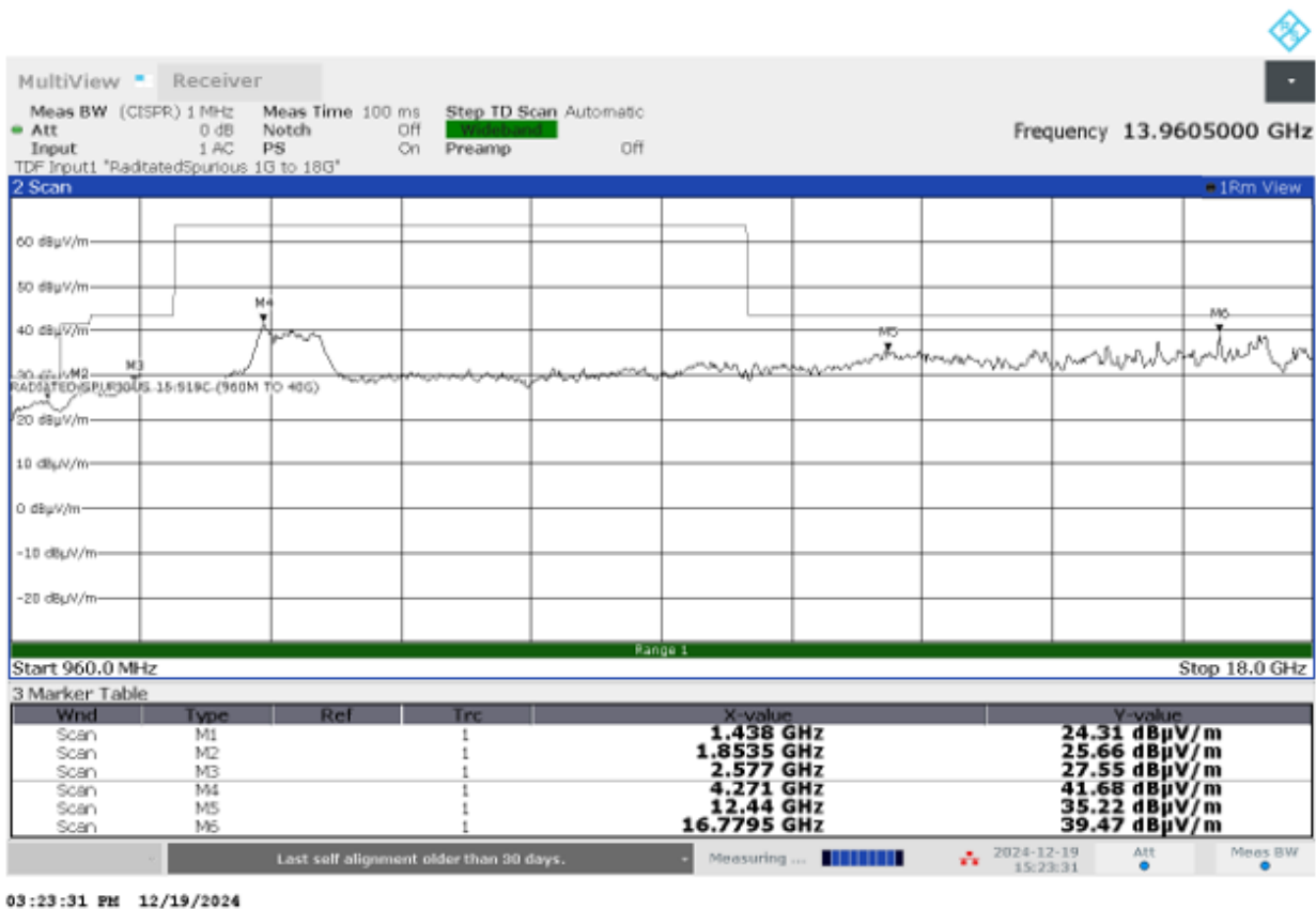
Figure 26. Radiated Emissions 960MHz – 18GHz (Vertical, Mid Channel)
