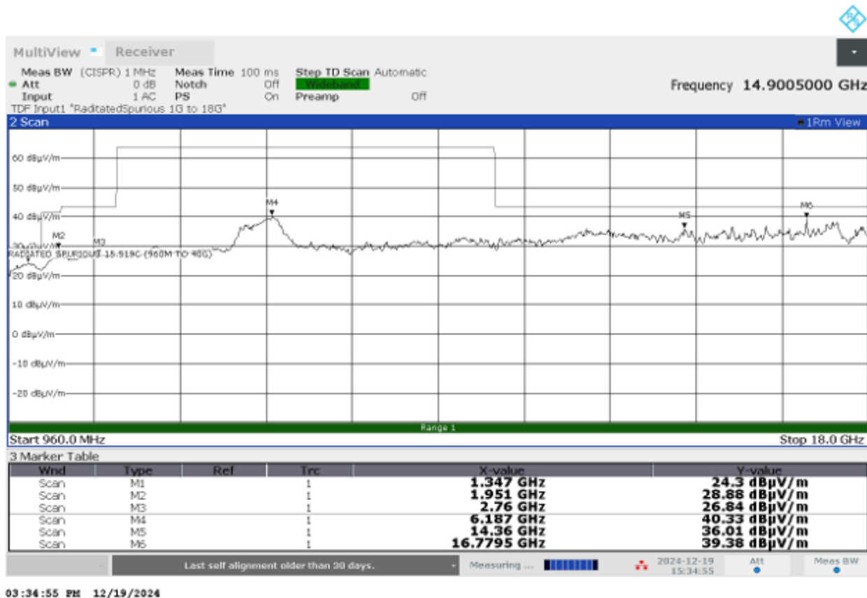
Figure 29. Radiated Emissions 960MHz – 18GHz (Horizontal, High Channel)
