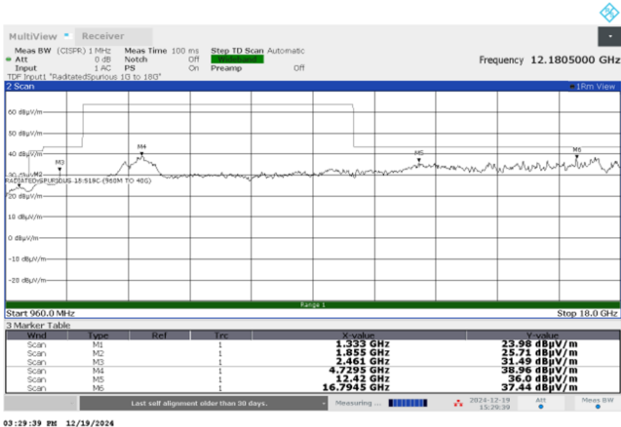
Figure 27. Radiated Emissions 960MHz – 18GHz (Horizontal, Mid Channel)
