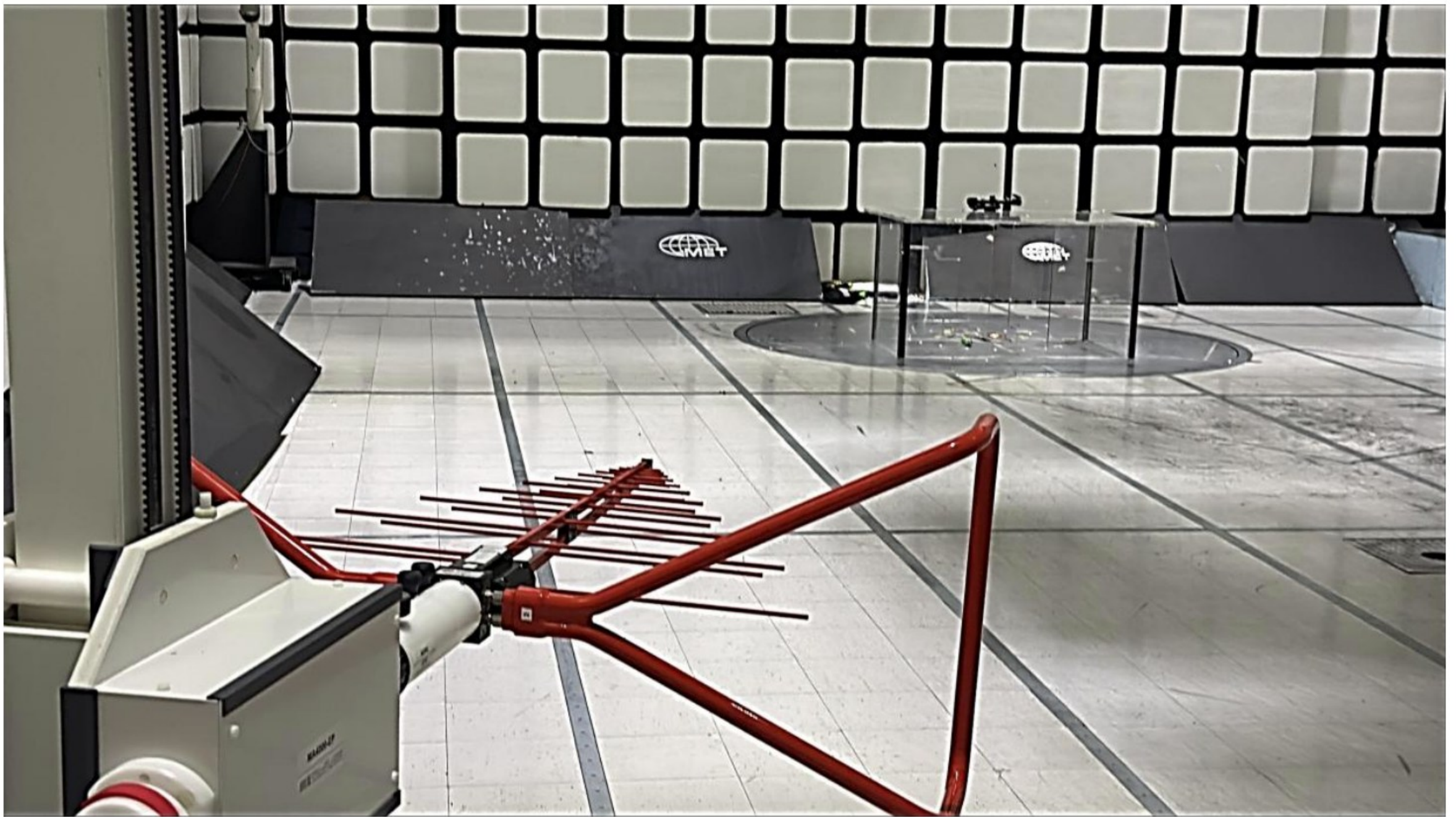
Photograph 3. Radiated Emissions, Lock, (30 MHz – 1000 MHz), Setup Antenna View
