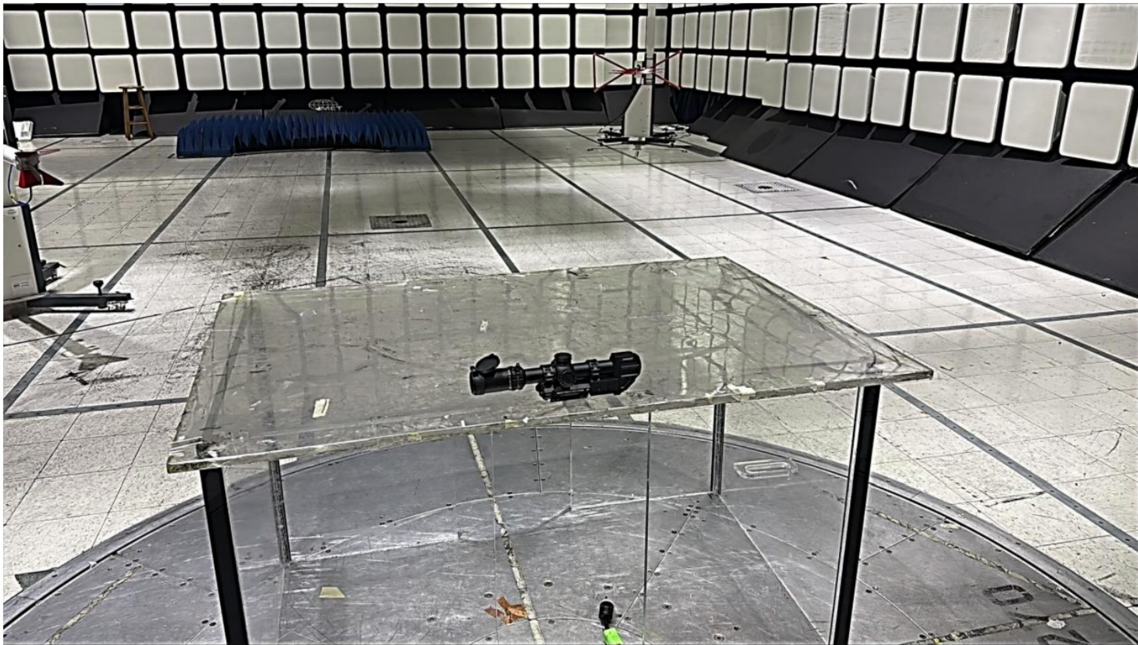
Photograph 2. Radiated Emissions, Lock, (30 MHz – 1000 MHz), Setup Rear View
