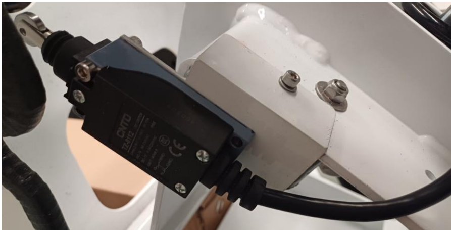
Figure 6: The “Deadman switch” engages when the pods are raised (stowed) to prevent inadvertent GPR transmissions.
