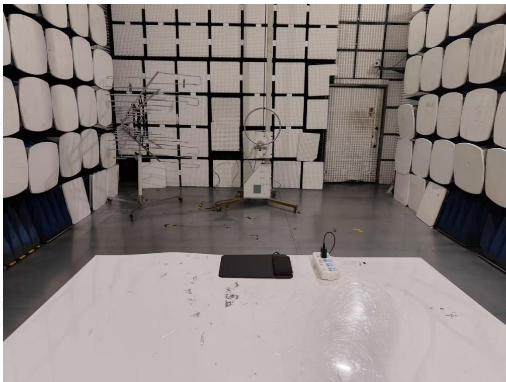
Radiated Emission below 30MHz-AC adapter charge mode
