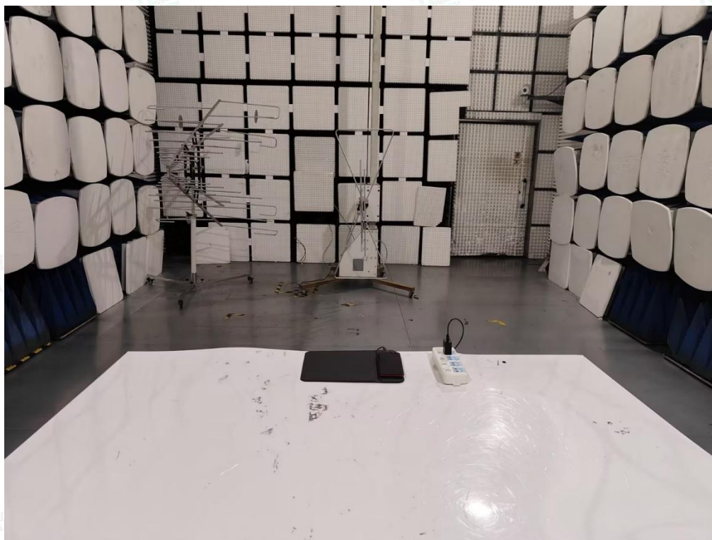
Radiated Emission below 1GHz-AC adapter charge mode
