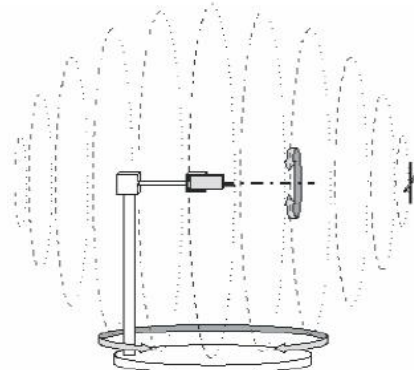
Figure (3) Three dimensional positioning device for mobile phone in darkroom
