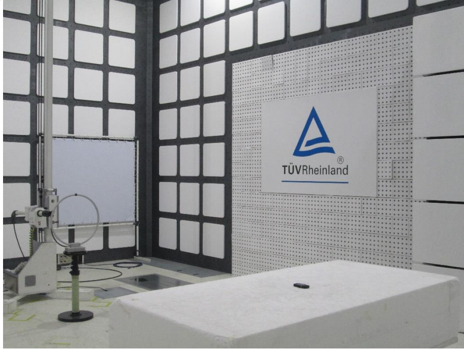
Photograph 4: Test Setup for Spurious Emissions (Back View 2)
