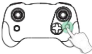
When the aircraft is flying, short press the (△) button, and the aircraft will automatically land on the ground
