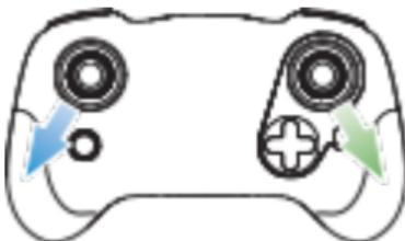
Simultaneously push the left joystick to the lower right corner and the right joystick to the lower left corner, the motor will rotate and the vehicle will be unlocked.
