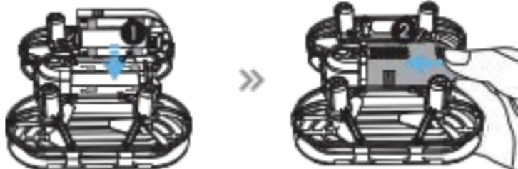
Installation: Install the battery onto the clips on the back of the craft as shown in the picture and push forward. Make sure the battery is securely installed.
