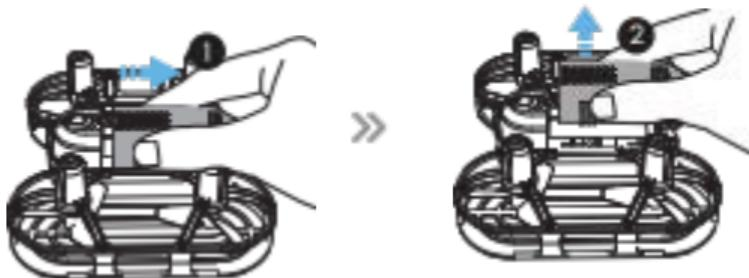
Removal: As shown in the picture above, pull the battery back by pressing on both sides, and then remove the battery upwards.
