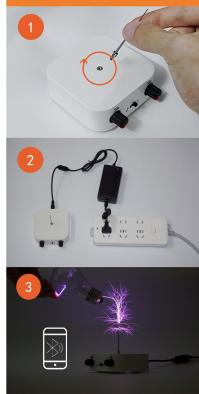
1. Install the discharge pin and turn the discharge pin clockwise until tightened
