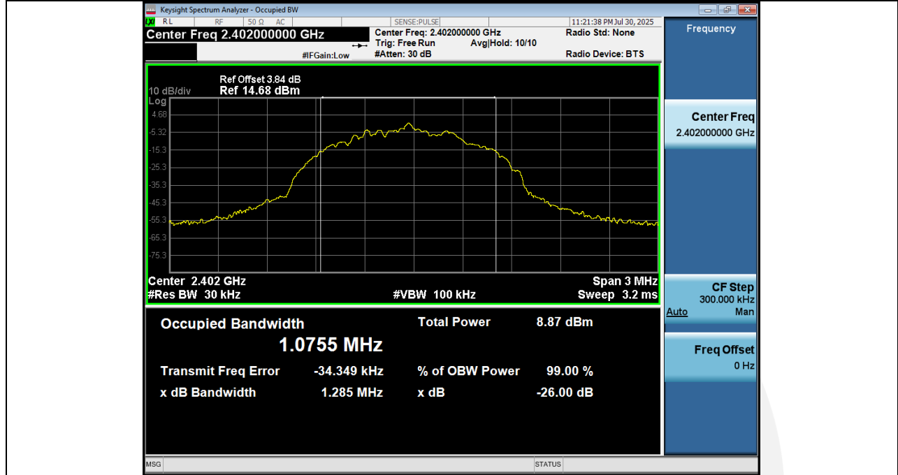
99% Occupied Bandwidth NVNT ANT1 1Mbps 2402
