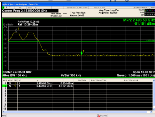
Out Of Band Emission(Right) GFSK_DH5_Channel Hopping
