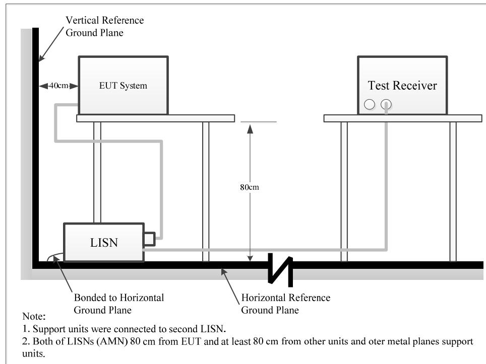
The setup of EUT is according with per ANSI C63.4-2014 measurement procedure. The specification used was with the FCC Part 15 B and Innovation, Science and Economic Development Canada ICES-003 Class B limits.
