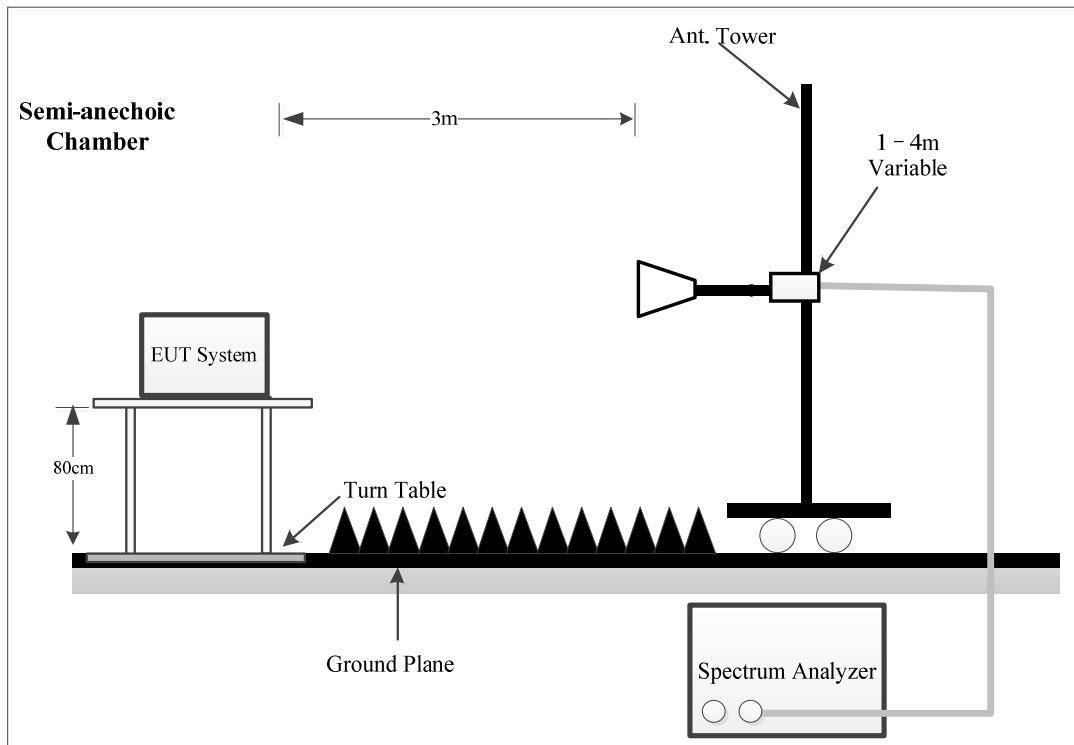
The radiated emission tests below 1GHz were performed at the 3 meters distance, above 1GHz were performed at the 3 meters Chamber B, using the setup accordance with the ANSI C63.4-2014. The specification used was the FCC Part 15B and ICES-003 Class B limits.
