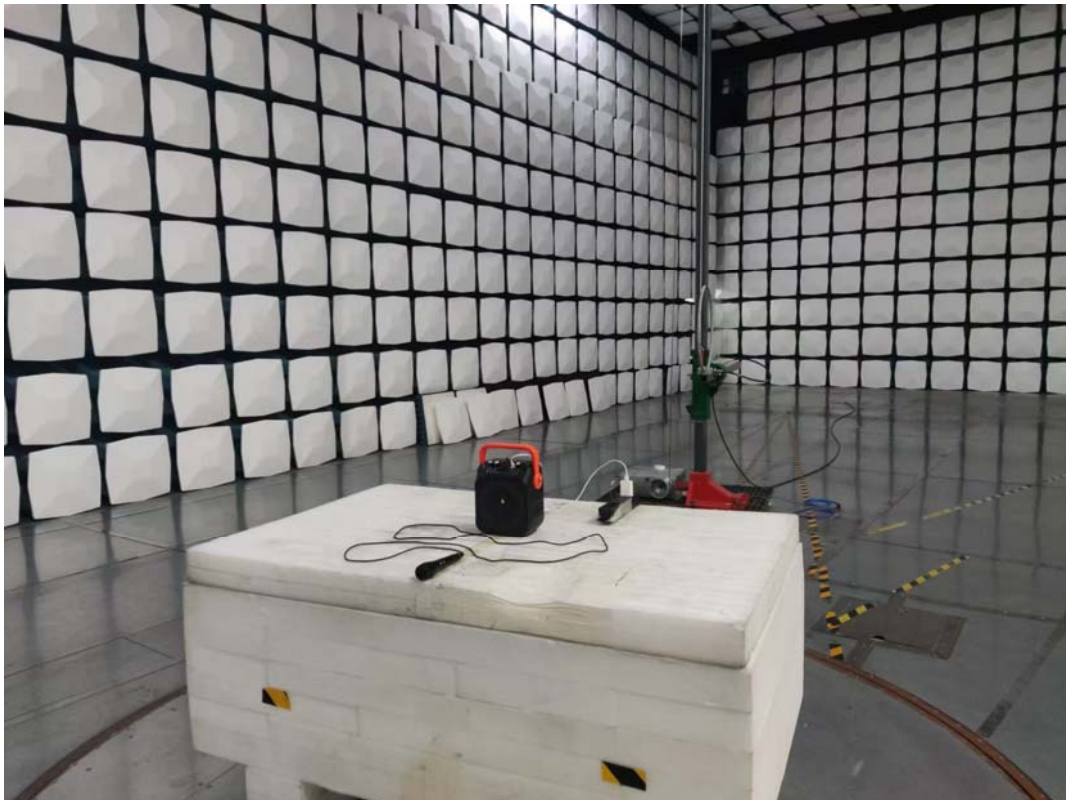
Radiated Emission 9k-30MHz Perpendicular View
