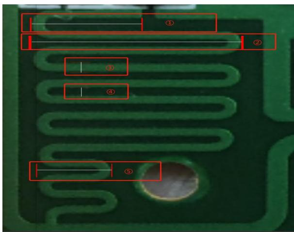
图标的尺寸：①、4.5mm ②、8.2mm ③、0.7mm ④、0.7mm ⑤、3mm
