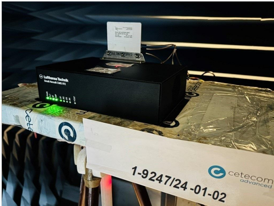
Photograph 3: EUT test setup in the fully anechoic chamber 2, close up view_EUT elevation 0°
