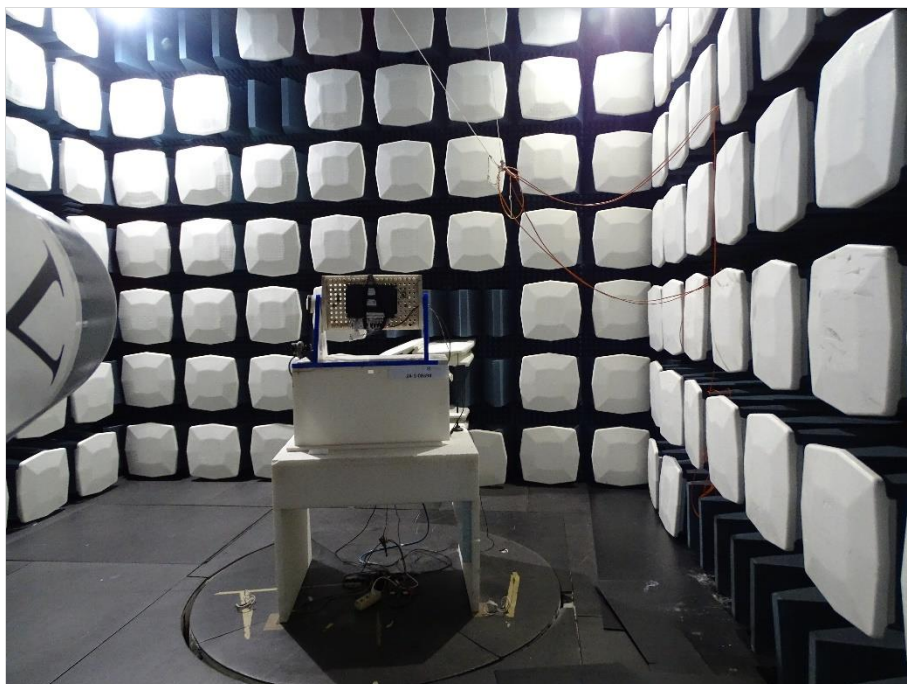
Photograph 6: EUT test setup in the fully anechoic chamber, overview_EUT elevation 90°
