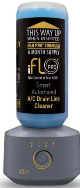
IFLOPROKIT01 mainly works together with HVAC system. The input of power source of device is wired to 24VAC low voltage output from HVAC secondary transformer. The input power source of the float switch interceptor cable is 24VAC as well to detect air conditioning drainpipe float switch event.
