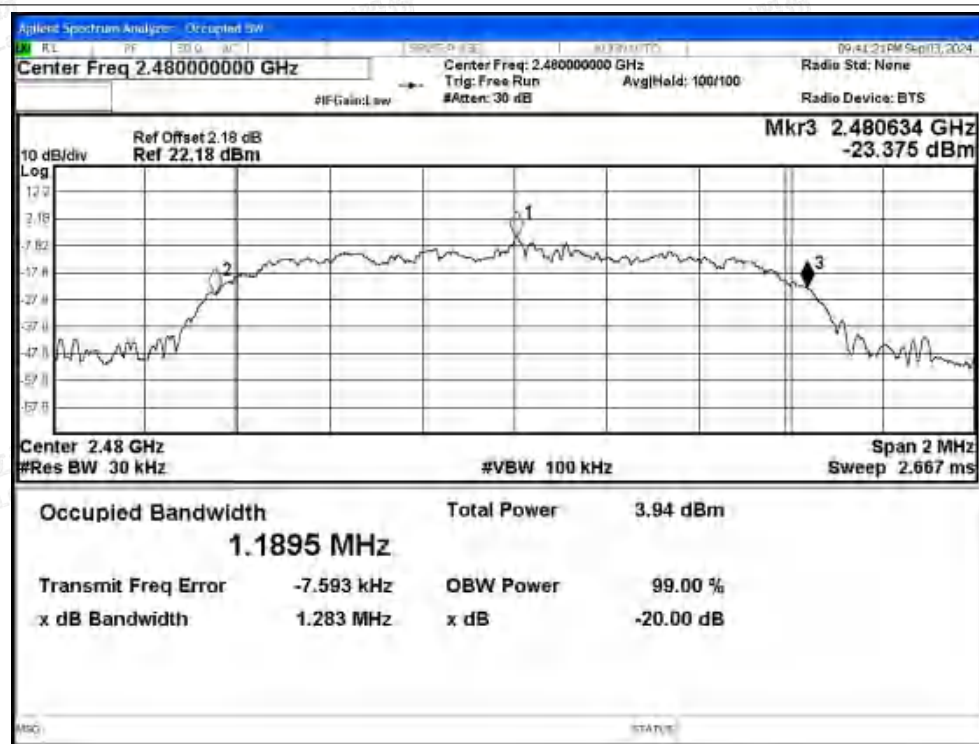
-20dB Bandwidth NVNT 2-DH5 2480MHz Ant1
