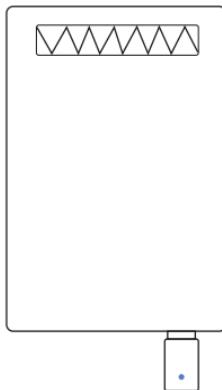
3.3.3 When the controller is not performing any operations and the receiver's indicator light flashes once every two seconds (slowly flashing), it indicates that the paired controller has low battery power, and it is recommended to replace the controller's batteries.
