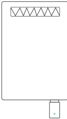
3.3.4 When the receiver has not been used for a long period, it will enter sleep mode. Once the controller goes to sleep, the corresponding USB indicator light will turn off while retaining the pairing information to facilitate a quick connection after waking up (if the USB receiver is powered off, the pairing information will not be retained, and it is recommended that customers check if the controller is connected after restarting).USB
