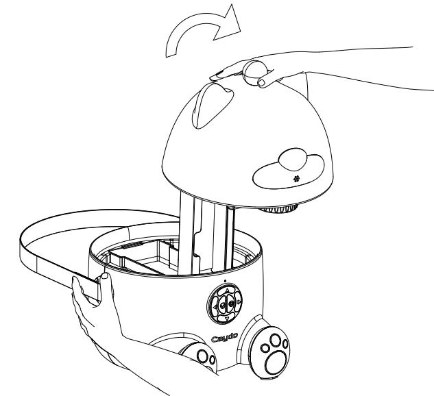
Hold the top of the projector steady and push from the back to the front until the stand is upright.
