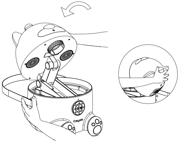
Hold the top of the projector steady and lift the top by pulling it from front to back.
