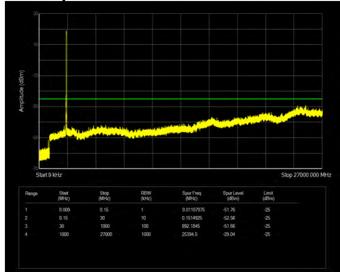
Band38 QPSK BW=15MHz Channel=38175 RB Size=75 Position=#0
