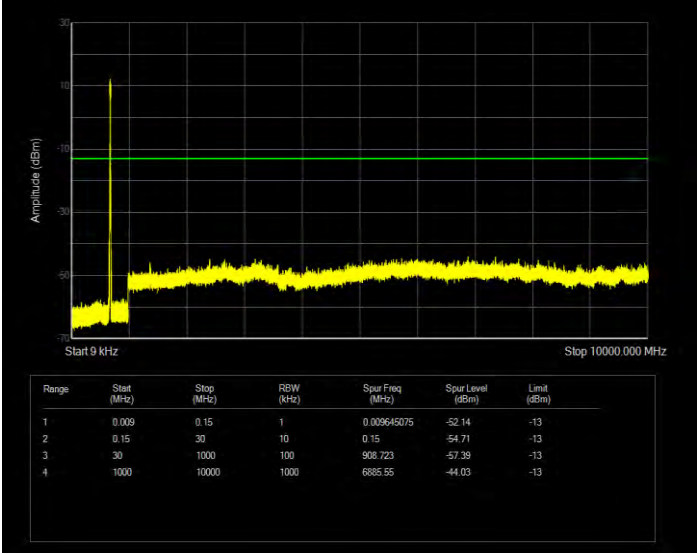
Band71 16QAM BW=10MHz Channel=133422 RB Size=50 Position=#0
