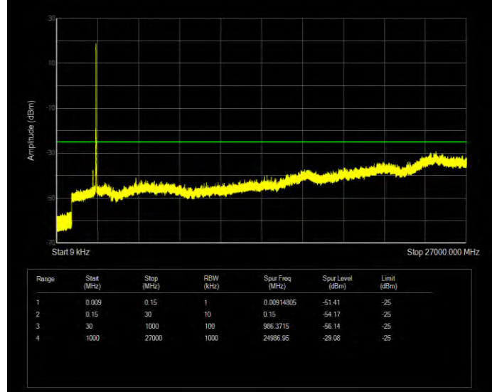
Band38 QPSK BW=20MHz Channel=37850 RB Size=100 Position=#0
