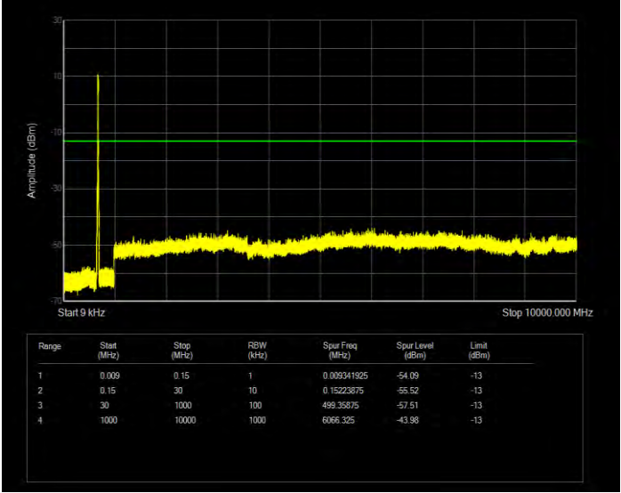
Band71 16QAM BW=15MHz Channel=133397 RB Size=75 Position=#0
