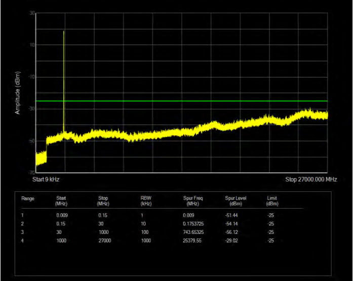
Band41(2535-2655) 16QAM BW=10MHz Channel=41190 RB Size=50 Position=#0
