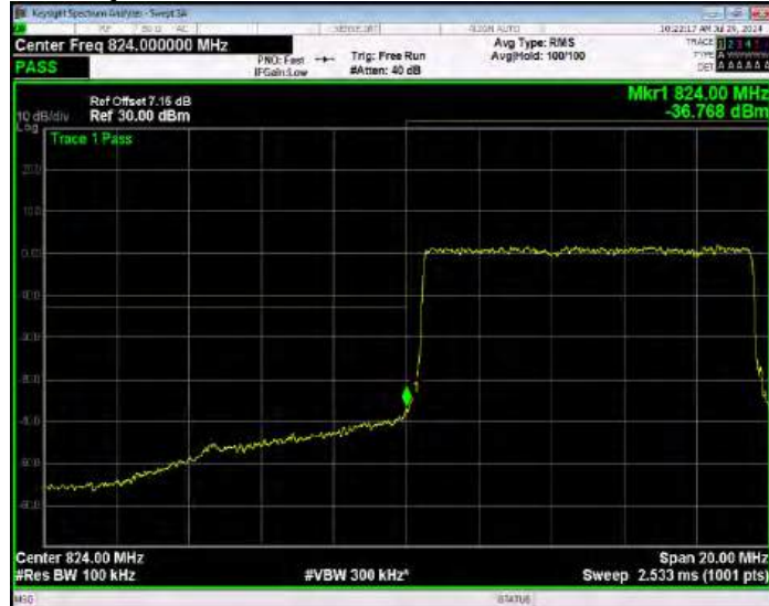
Band5 16QAM BW=10MHz Channel=20450 RB Size=50 Position=#0 Normal
