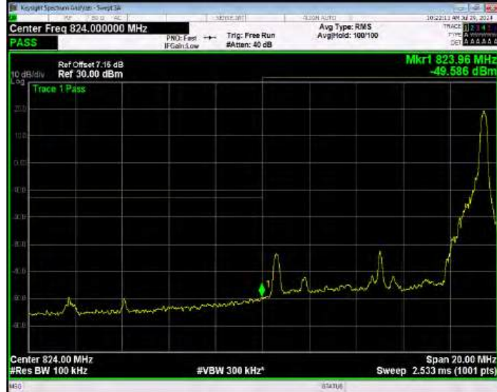
Band5 16QAM BW=10MHz Channel=20450 RB Size=50 Position=#0 Extended
