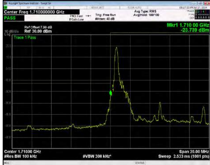
Band4 16QAM BW=10MHz Channel=20000 RB Size=1 Position=#Max Extended
