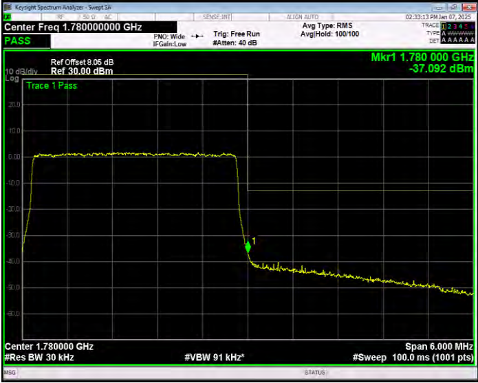
Band66 16QAM BW=3MHz Channel=132657 RB Size=15 Position=#0 Normal
