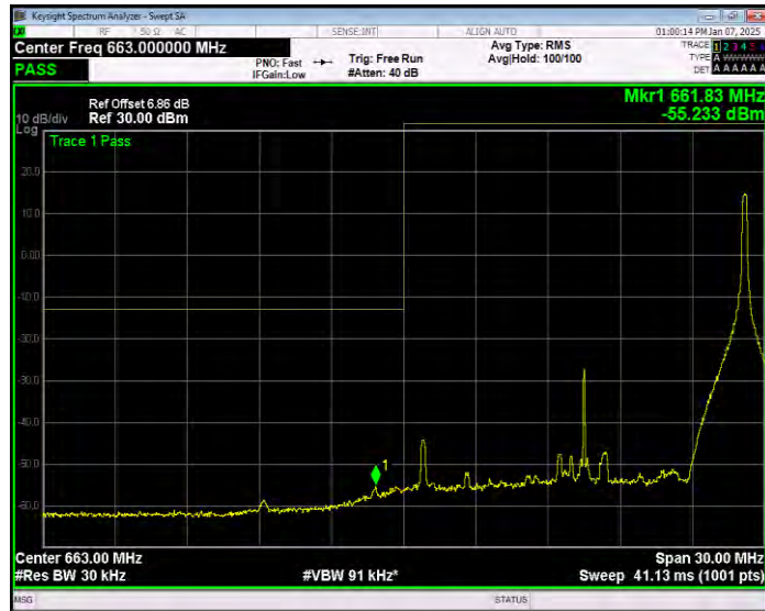
Band71 16QAM BW=15MHz Channel=133197 RB Size=75 Position=#0 Extended
