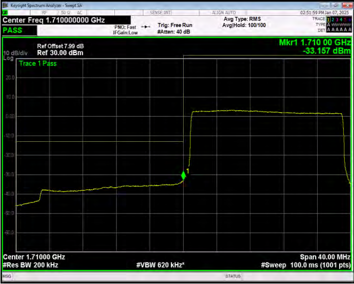
Band66 QPSK BW=20MHz Channel=132072 RB Size=100 Position=#0 Normal
