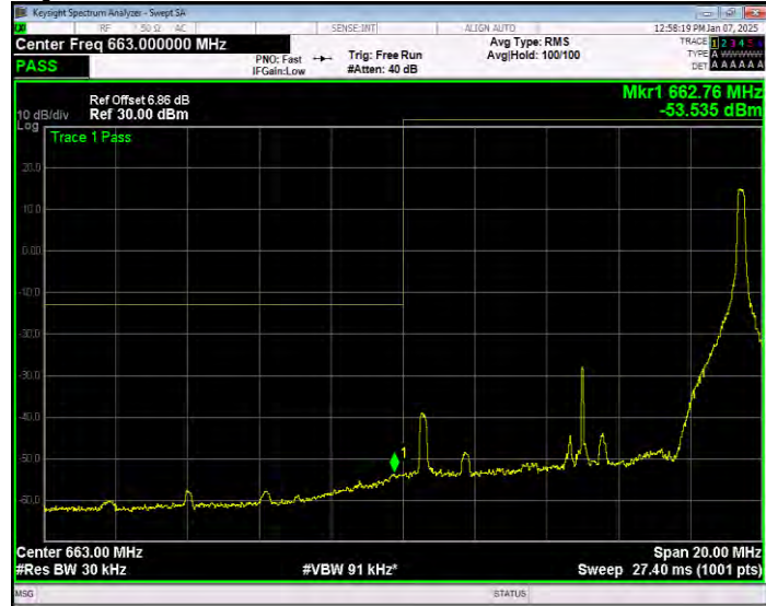
Band71 16QAM BW=10MHz Channel=133172 RB Size=50 Position=#0 Extended
