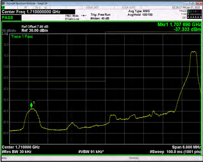
Band66 16QAM BW=3MHz Channel=131987 RB Size=15 Position=#0 Extended
