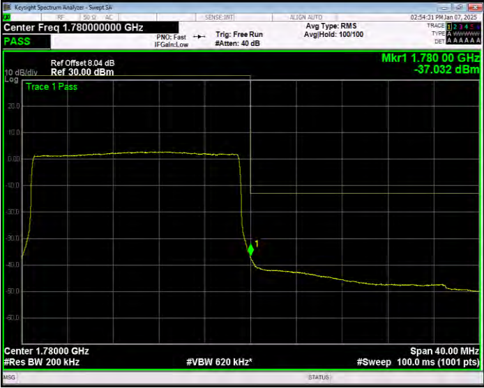
Band66 QPSK BW=20MHz Channel=132572 RB Size=100 Position=#0 Normal
