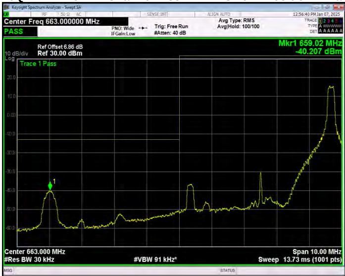
Band71 16QAM BW=5MHz Channel=133147 RB Size=25 Position=#0 Extended
