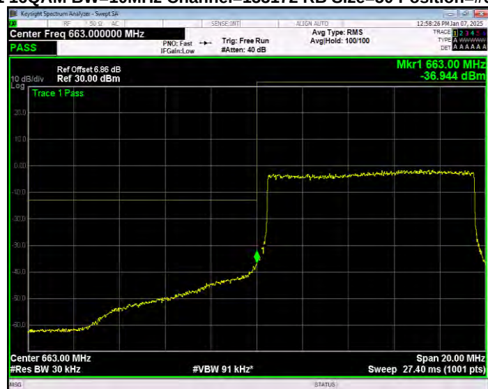
Band71 16QAM BW=10MHz Channel=133172 RB Size=50 Position=#0 Normal
