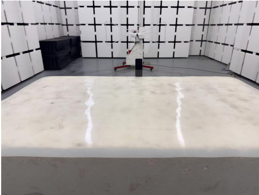
Set-up for Radiated Spurious Emission, Above 1GHz
