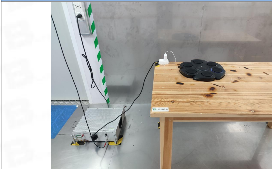
Conducted Emission at AC power line
