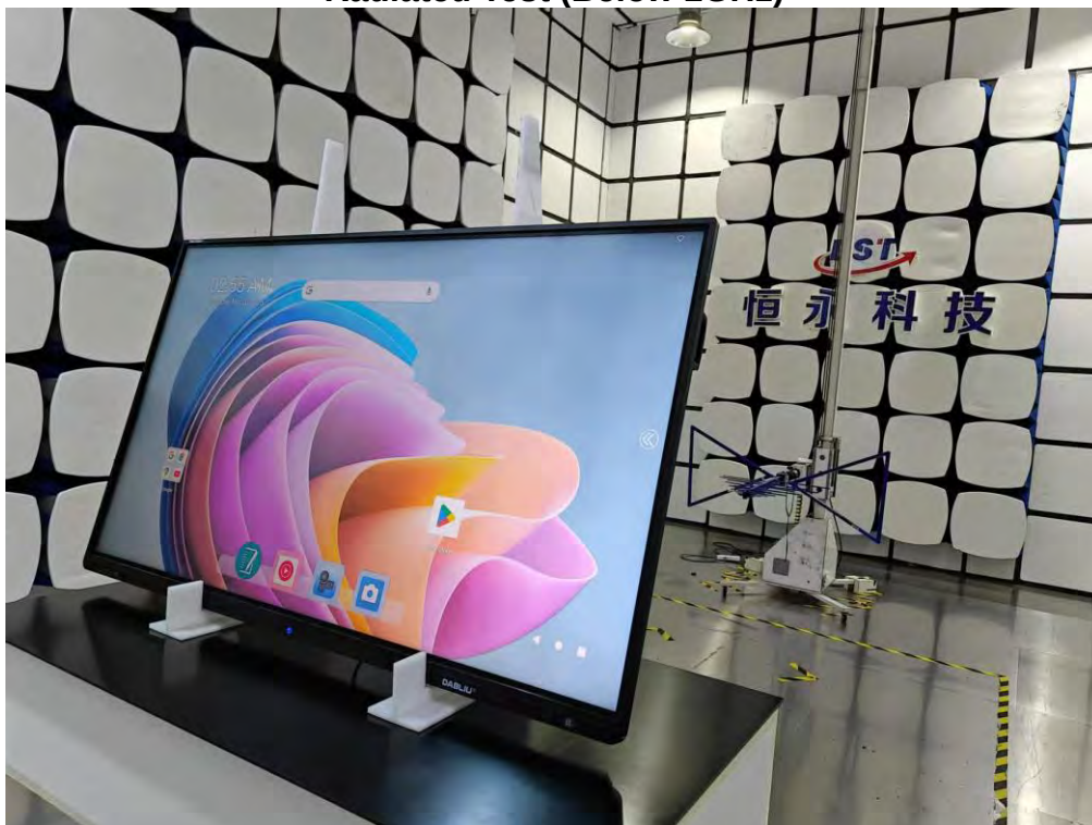
Radiated Test (Below 1GHz)
