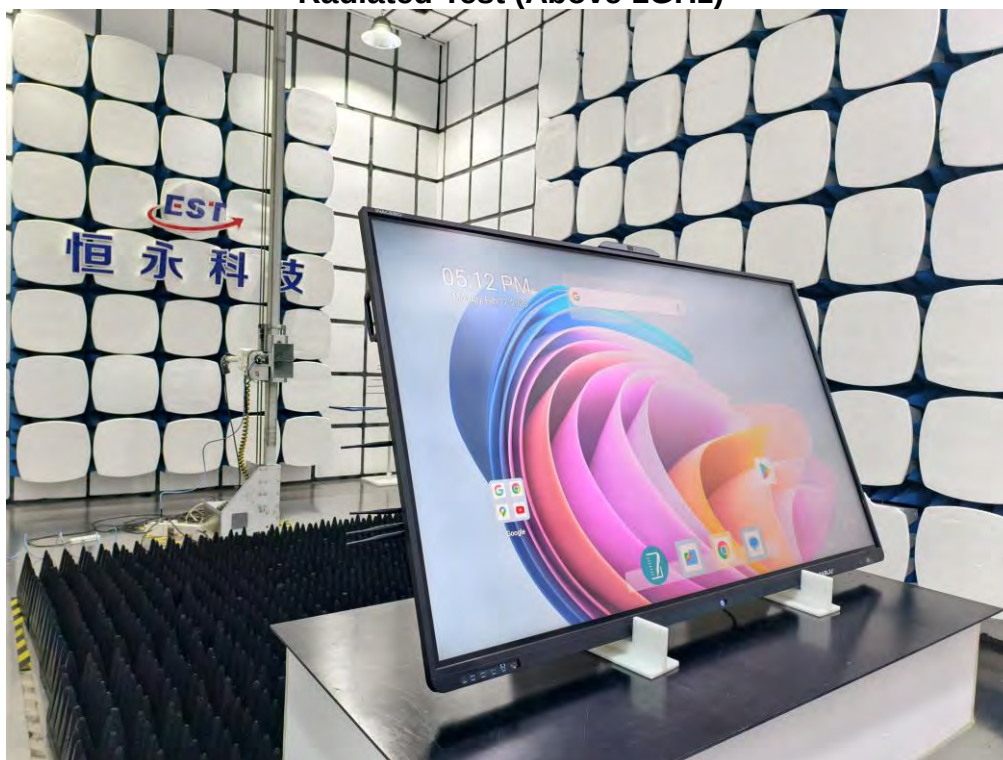
Radiated Test (Above 1GHz)
