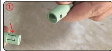
Hold down the part of the arrow with your hand, and then slip the other end into the power connector
