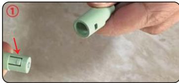
Hold down the part of the arrow with your hand, and then slip the other end into the power connector
